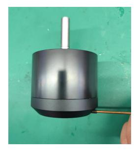
The locking screws on both sides need to be removed.
