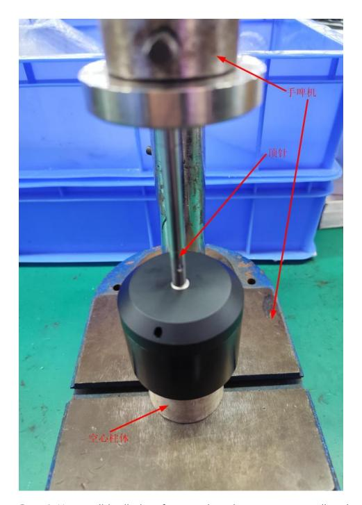
**Step 4:** Use a solid cylinder of appropriate size as a support, align the shaft locking screw hole with the rotor screw hole, and use a hand press to press the new shaft into the rotor until the shaft is flush with the rotor end face, as
