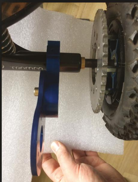
**ATTENTION :** LES TRUCKS MOUNTS POUR VERTIGO SONT ASYMETRIQUES, IL Y A UN DROIT ET UN GAUCHE, VOUS NE POUVEZ LES INTERVERTIR, CELA EST VISIBLE DANS L'EMPREINTE DU MOUNT QUI SUIT L'EVOLUTION DE LA SECTION DU TRUCK
